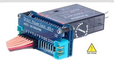
The **PowerJack 6014** is a 14 channel Servobox with double buffered voltageregulators for the 6014 type receiver. It is directly plugged onto the 6014 by precision jacks. Two high current MPX-connectors can be connected with one or two batteries by a power-switch harness.
