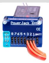
The **PowerJack 6X8** is a 8 channel Servobox with buffered voltageregulator for the 6X8 family receivers. It is directly plugged onto the 6X8 by precision jacks. A high current MPX-connector can directly be connected with a battery by a power-switch harness.
