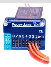
The **PowerJack 7009** is a 8 channel Servobox with buffered voltageregulator for the 7008SB (6308SB) family receivers. It is directly plugged onto the receiver by precision jacks. A high current MPX-jack can directly be connected with a battery by a power-switch harness.
