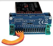
The **PowerJack 7014** is a 14 channel Servobox with double buffered voltageregulators for the 7014 type receiver. It is directly plugged onto the 7014 by precision jacks. Two high current MPX-connectors can be connected with one or two batteries by a power-switch harness.
