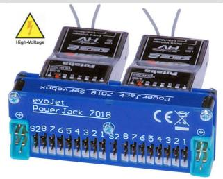
The **PowerJack 7018** is a 16 channel Servobox for a double 7008SB (6308SB) family receiver set. They are directly plugged onto the 7018 by precision jacks. Two high current MPX-jacks can be connected with one or two batteries by a power-switch harness.
