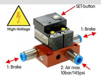
The evoJet **PRO-Proportional** – **brake valve** is made for wheel-brakes using compressed air. For a scale-like and controlled braking the valve uses proportional air dosage. A double working valve technique (fill or drain) needs just a minimum amount of compressed air (low loss).
