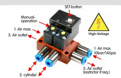
The evoJet **PRO-HV Double-Action-Valve** is made for double working air cylinders. Where both the extension and retraction of the landig gear or flaps are powered by compressed air.
