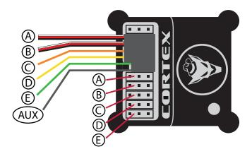
Channels that are not subject of being stabilised, e.g. gas, must not be looped through, but must remain connected directly to the receiver.
